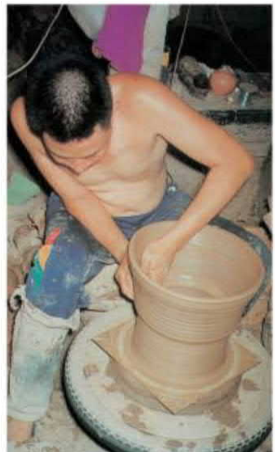
A potter's wheel is a major tool used in forming the shape of a piece of pottery
