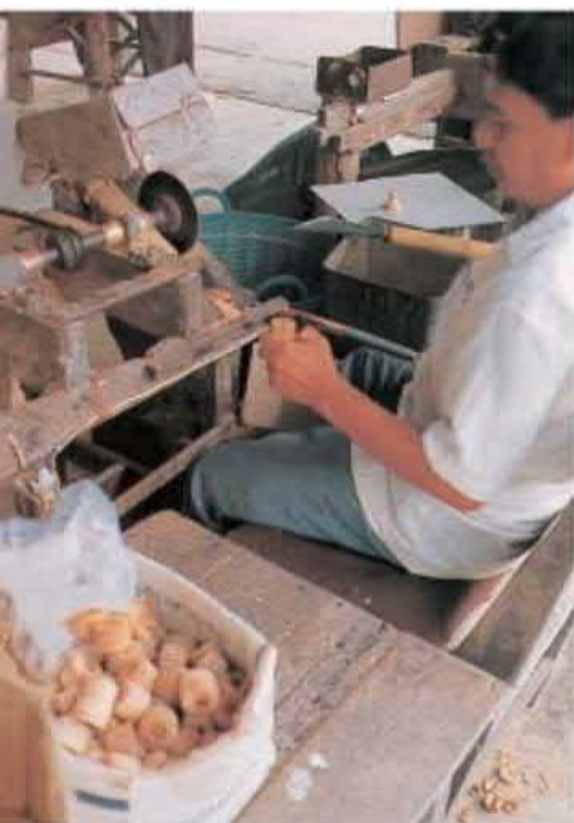
Making a knob and a hub with a lathe
