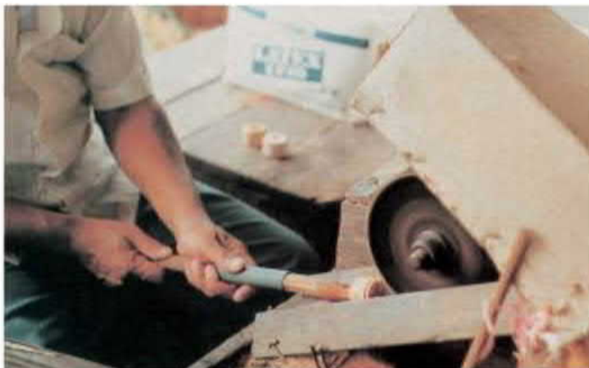
Cutting the hub into grooves. The number of the grooves matches the number of the spokes attached to the umbrella
